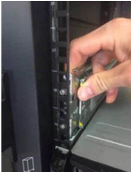
Front rack post attachment details
