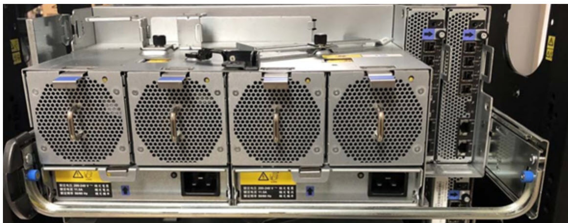
Crossbar with blue thumbscrews stabilizes the two rails at the rear of the chassis
