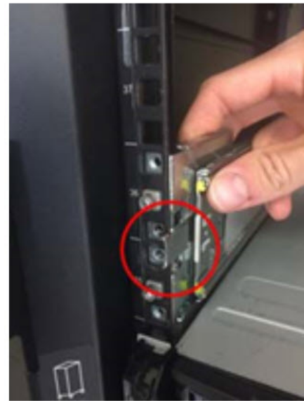
Front rack post attachment details
